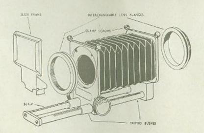
Fitting the unit to the camera. There are two methods of fitting the unit to your camera. The conventional way is to remove the lens from the camera and screw the unit in its place by turning the complete assembly round until it is fully screwed home into the camera front, then release the small knurled screws which allow you to adjust the unit and re-lock square with the camera body. The lens is then screwed into the front panel of the bellows unit.
