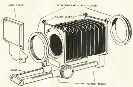
**TELEPHOTOGRAPHY.** Extra mounts can be made to suit non-standard lenses. This will allow lenses from old film or plate cameras to be used as long focus lenses. Any 3in, to 6in, lens without any means of focussing is suitable. The bellows becomes a focussing mount. Telephoto magnification can be found by dividing standard lens into focal length of long focus lens.
